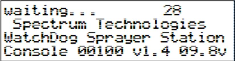
The bottom line of the startup display contains (from left to right) the Console Serial Number, the firmware version number, and the initial voltage level of the internal battery, or the external power supply (if connected).
