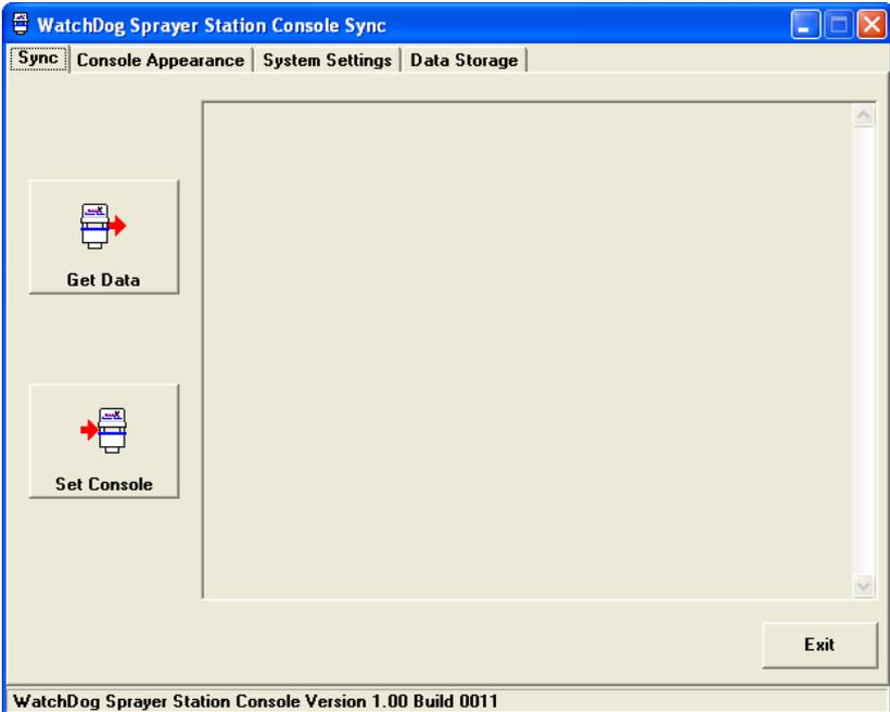
Before using either button on the Sync tab, you must connect your Console to the PC using the black PC Interface cable. See **System Settings** (p. 21) for more details.
