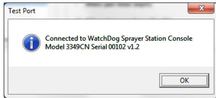
Select the serial port to be tested and click on the **Test Port** button. If the message “Connection OK” is displayed, another device (such as a modem) is probably connected to that port. If the message “No Connection” is displayed, this port may be the one connected to your serial cable and you can proceed to the next step.
