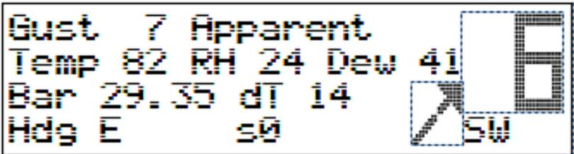
The above screen shows weather data without GPS information. In this case, the word "Apparent" appears in the top line. This will be displayed until the GPS obtains a position fix. The GPS time to first fix is approximately one minute. Note that a GPS fix will not be possible when there is not a clear view of the sky. This would be the case indoors or in a heavily forested location.
