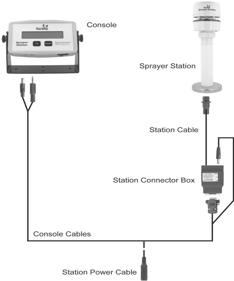
bracket. Mount the Console bracket securely with bolts, screws, foam mounting tape, or Velcro strips. Put the Console back in the bracket and tighten the side knobs. You may wish to secure the cables that plug into the console. Because the Console will periodically be removed from the cab to transfer weather data to your PC, avoid having the cables fall to the floor.
