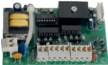
The 8 way input board allows 8 switched inputs to control a Heron irrigation controller.
