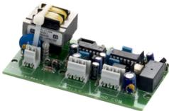
The level sensor board allows level sensing in a water tank using stainless steel rods.
